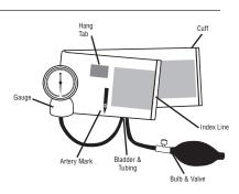
Most models come preassembled and ready for use. If assembly is required, attach gauge and bulb and valve assemblies to the tubes as shown in illustration. To facilitate, use alcohol or soapy water.
