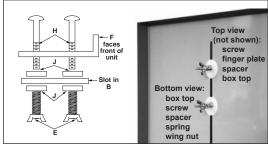
FIGURE 3 Slide Device Assembly
