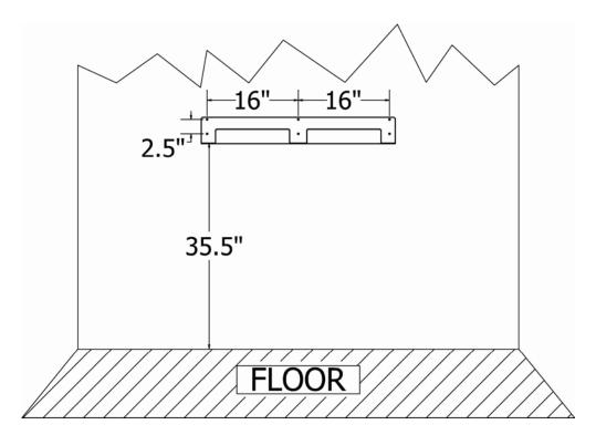
The wall mount allows the scale to be adjusted up or down and left or right to accommodate floors that may not be perfectly flat. This insures the accuracy of the weighing platform and prevents undue stress to the scale.
