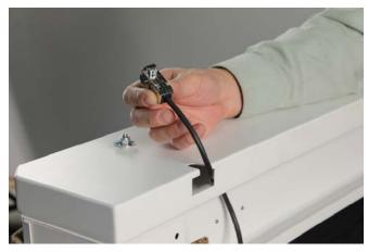
**4.** Continue feeding the load cell cable through the scale frame and up through the notch in the top of the scale frame.
