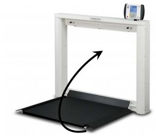
Lift weighing platform up to return to the closed (stored) position.
