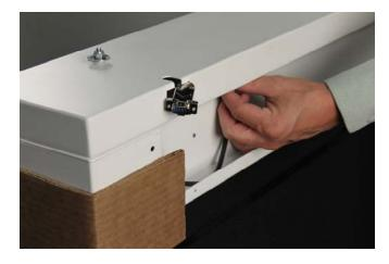
**3.** Feed the load cell cable through the large cut-out in the back of the scale frame.
