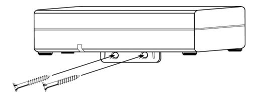
4. Tighten the screws to secure the display bracket to the wall.
