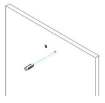
3. Place the display against the wall and insert the two (2) screws through the holes in the display bracket and into the wall anchors.
