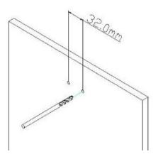
2. Insert the wall anchors in the wall until they are flush with the wall.
