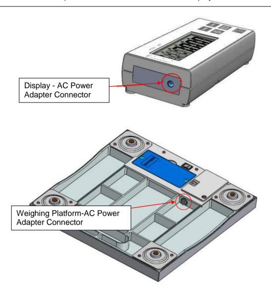
The scale's weighing platform and wireless display require separate electric power. Before using the scale, please make sure that both the scale base and wireless display have batteries correctly installed or both adapters correctly plugged in.
