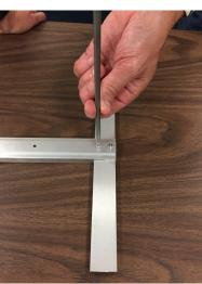
Obtain the two black end caps from the clear bag. Attach them to the ends of the footpiece. The front of the end cap should be flush with the front of the height rod.
