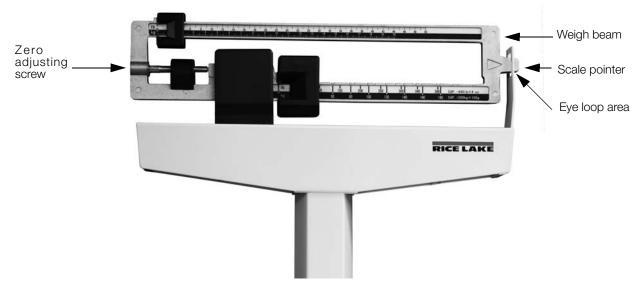
Figure 3-1. Eye Loop Area and Zero Adjusting Screw Location (Lb and kg version without height rod shown)
